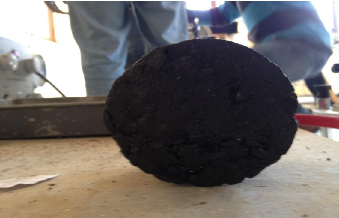
Fig 4.7 Failed Sample with Lateral Elongation
