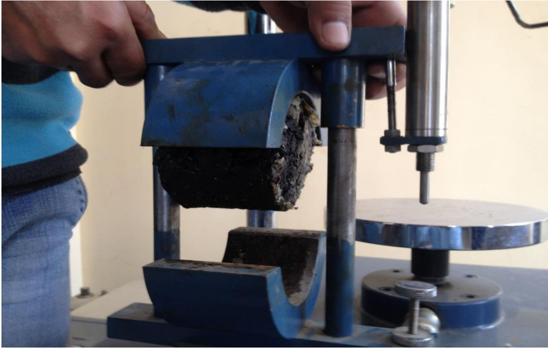
Fig 4.6 Removing the sample from the Apparatus after Load Test
