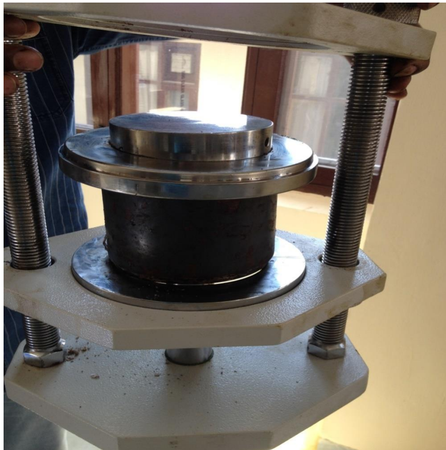
Fig 4.1 Extraction of Sample from the Mould for Testing
