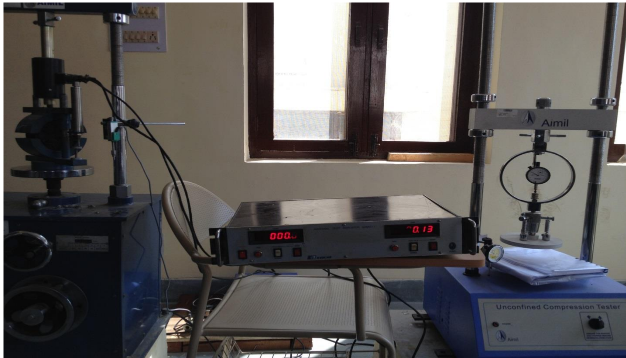
Fig 4.5 Performing Marshall Stability and Flow Value Test
