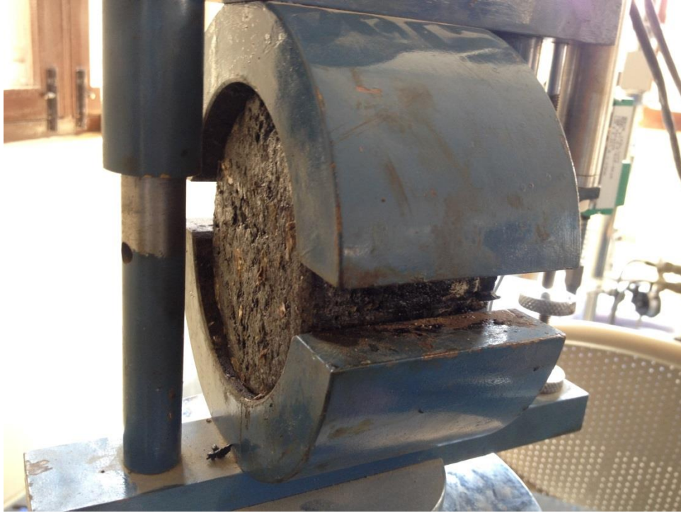
Fig 4.3 Sample placed in Marshall Stability Test Apparatus
