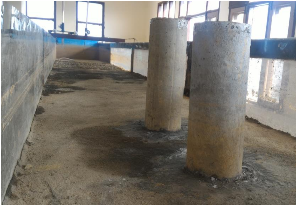
Fig 3.3 Piers at a stream wise spacing equal to three times of pier size
