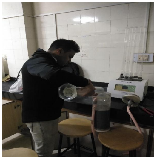
Figure 3.16 Pouring of chemical solution into prepared soil sample
