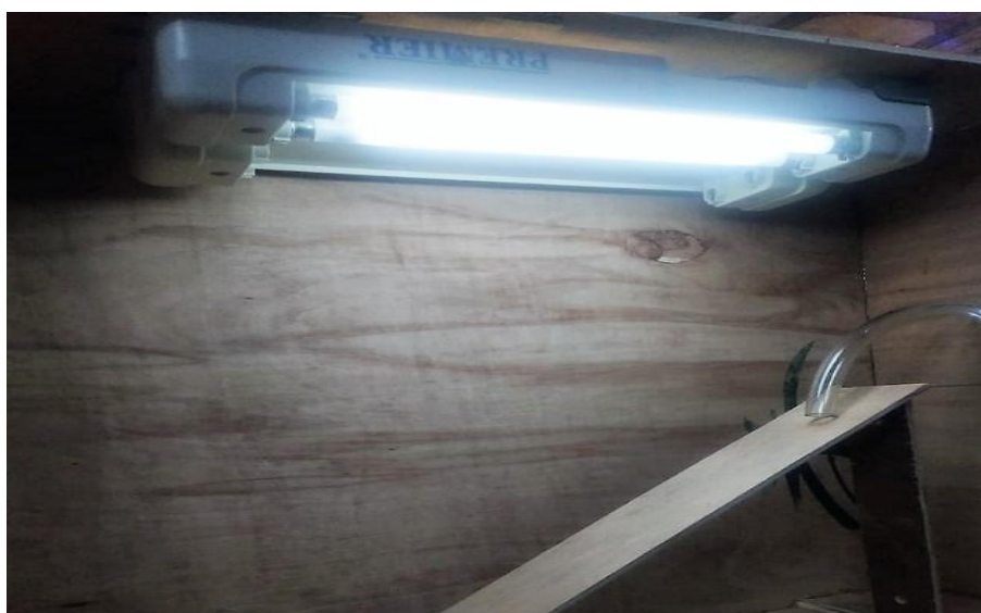
Figure 3.11 UV-lamp setup inside reactor
