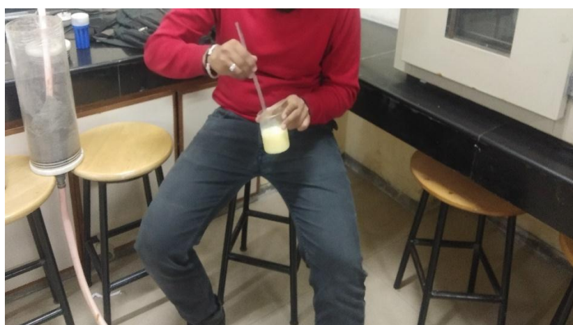
Figure 3.13 Gradually mixing of TiO 2 to avoid formation of lump
