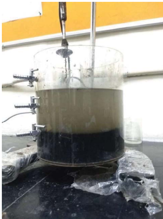
Figure A.4 Settling of Sludge
