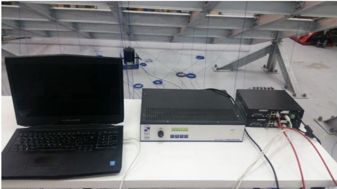
Figure 6.4: Data acquisition devices, modal shaker's amplifier
