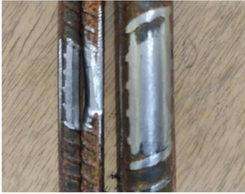
Figure 3.11: Rebar specimen prepared For bonding
