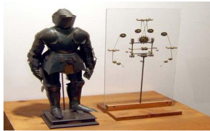
Figure 2: Leonardo da Vinci model of a Humanoid Robot with its Internal Mechanisms
