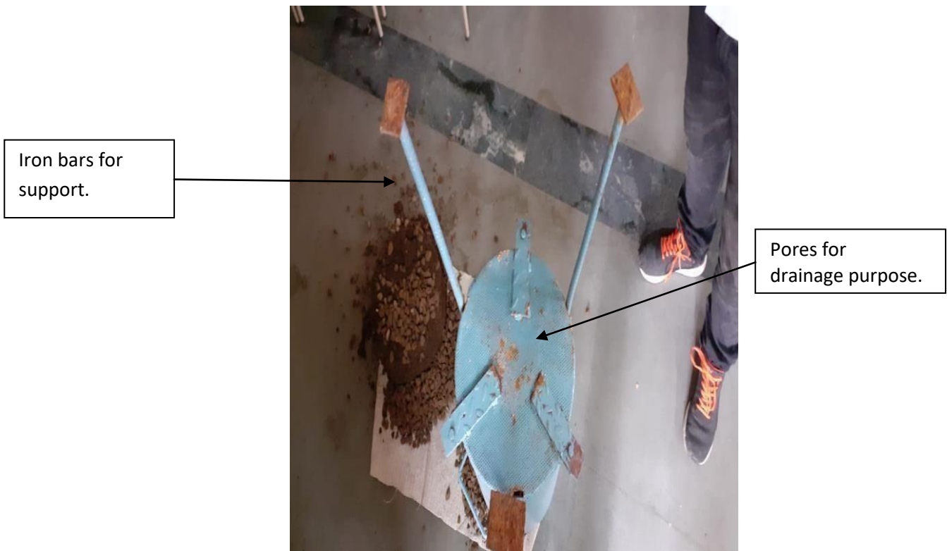
Figure 5 Leachate model drainage view
