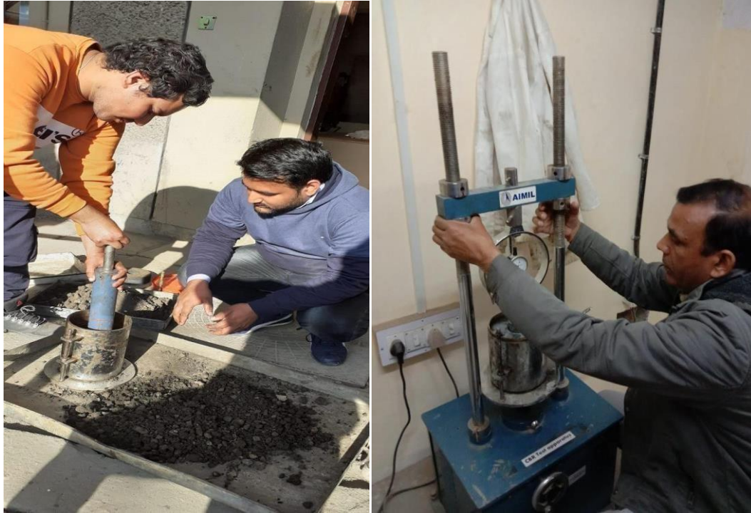
Figure 9 Compacting the soil and CBR test machine
