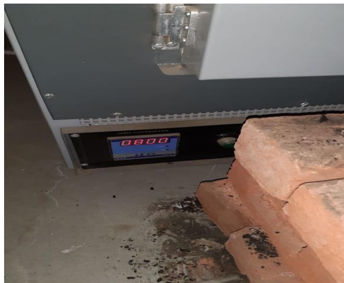
Figure 5 Incinerator burning at 800°C
