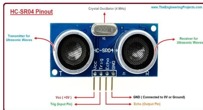
Fig 4.2: Ultra sonic Sensor
