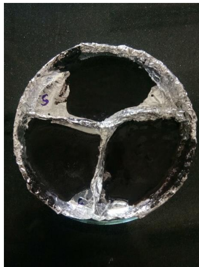
Fig 4.6: Bioplastic Films using glycerol, pectin, starch, cellulose
