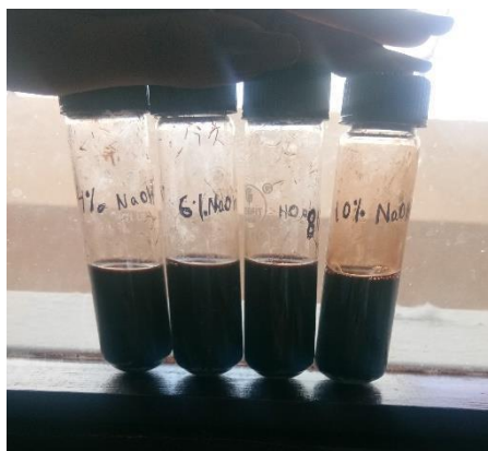
Fig 4.1: NaOH showed the best dissolution of hair
