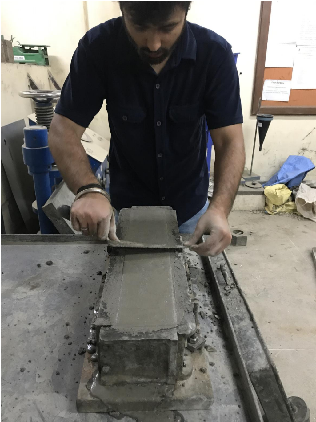
Figure 3.3: Preparing of specimen For Flexural Strength
