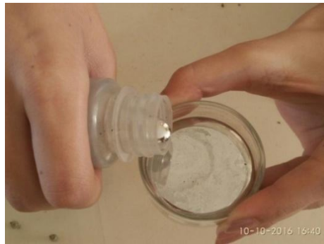
Fig. 10 - Mercury used for measuring volume of dry soil pat
