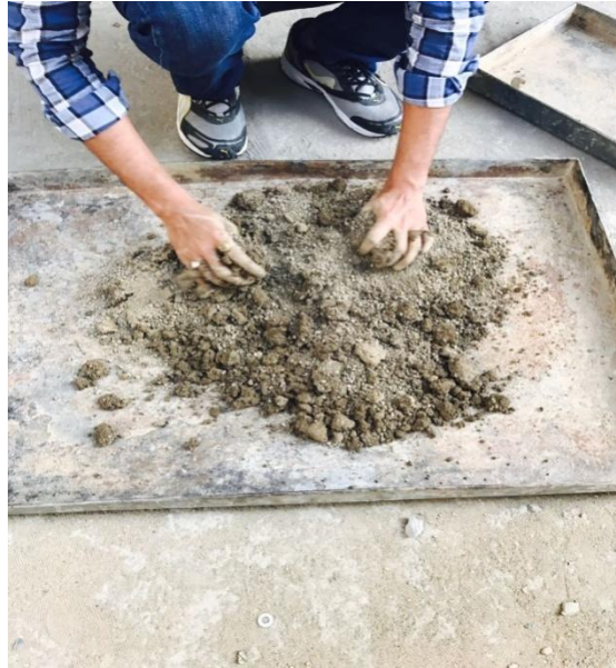
Fig 14- Preparation of sample for CBR test on unsoaked soil
