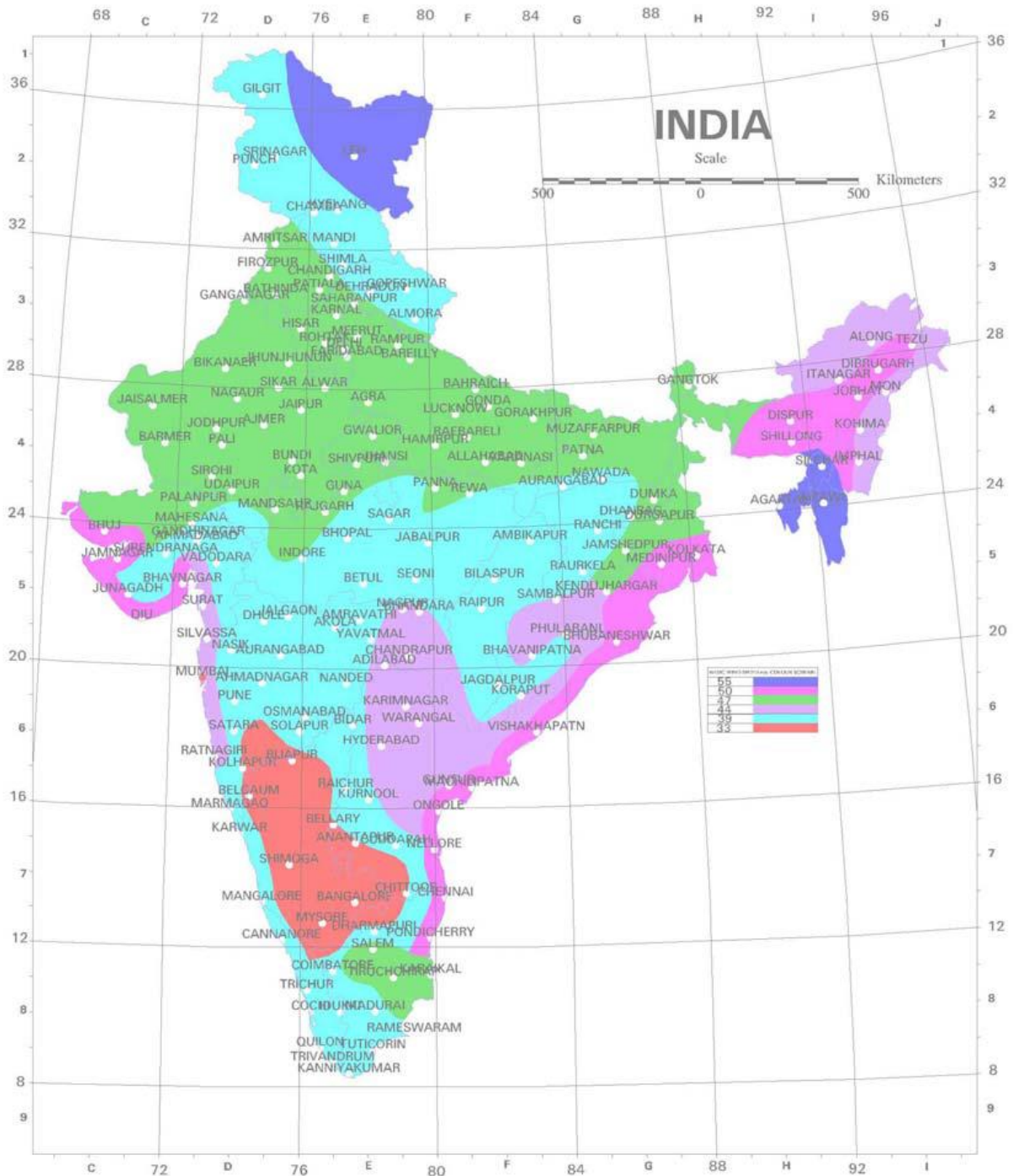
Figure no. - 12: Basic wind speed in m/s (based on 50 year return period)
