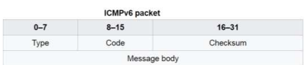
Fig 2.2 ICMPv6 packet format
