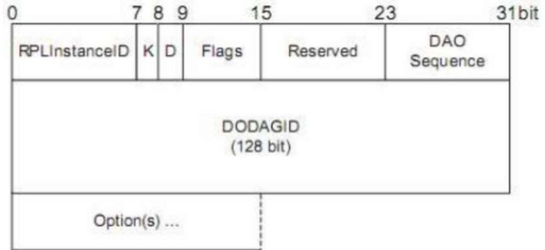
Fig 2.9 DAO Message Structure
