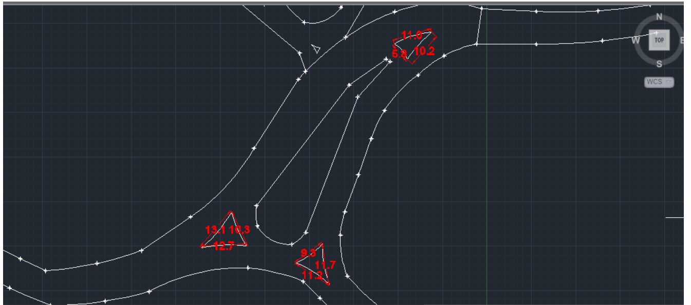
FIGURE 8 CHANNELISING ISLANDS WITH THEIR DIMENSIONS
