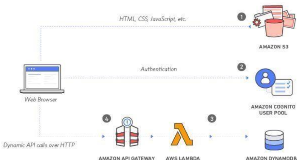
Fig 6.1: Deployed Website Architecture
