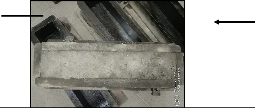
Fig 3.1: Preparation of steel reinforced beam specimen (type I)
