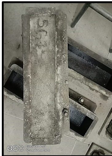
Fig 3.3: Preparation of sand-coated GFRP reinforced beam specimen (type III)
