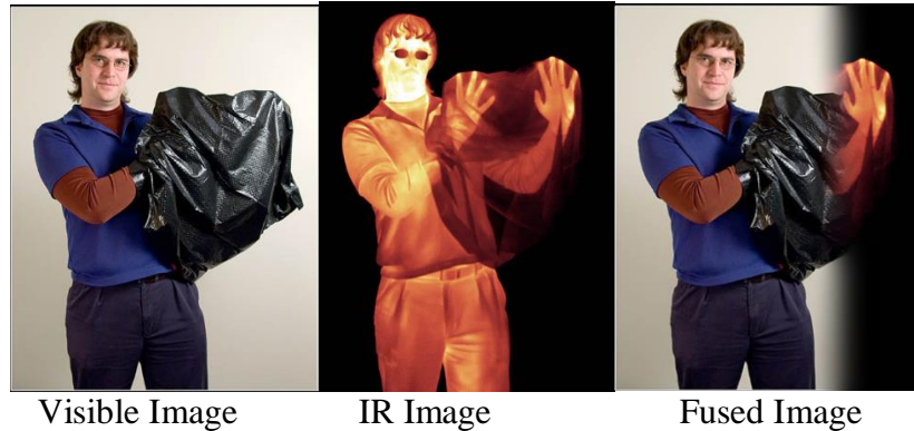
Fig. 15 : Image fusion of Multispectral images using Laplacian Pyramid
