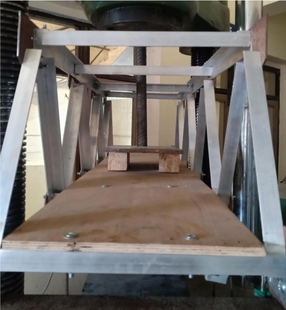
Figure 3.23 Image of Load Imprint provided on the deck of bridge prototype
