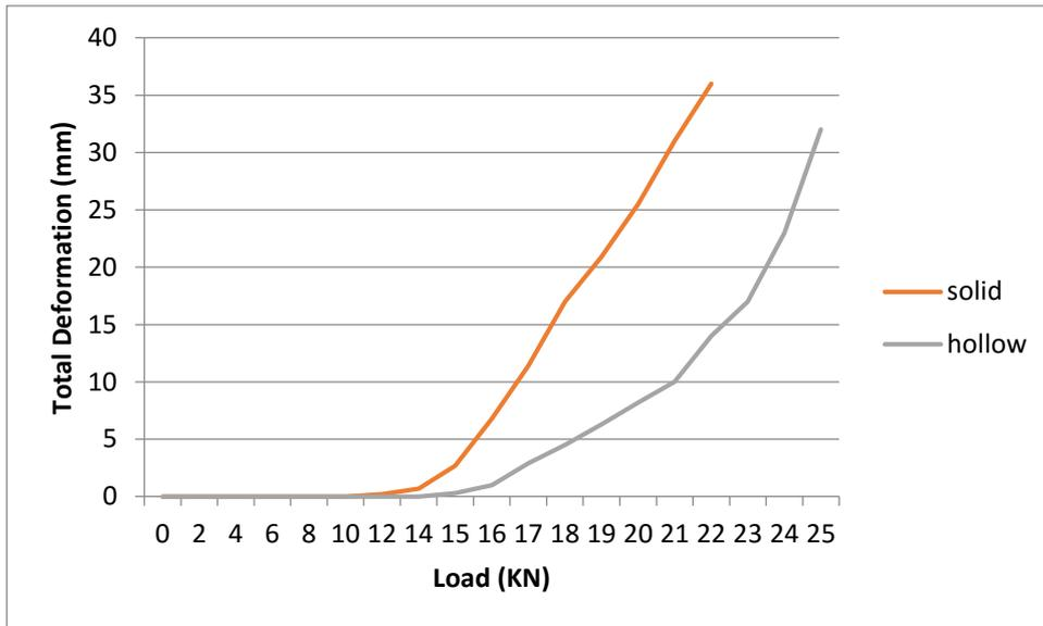
**Figure 4.8** Deformation comparisons at node 1 with respect to load
