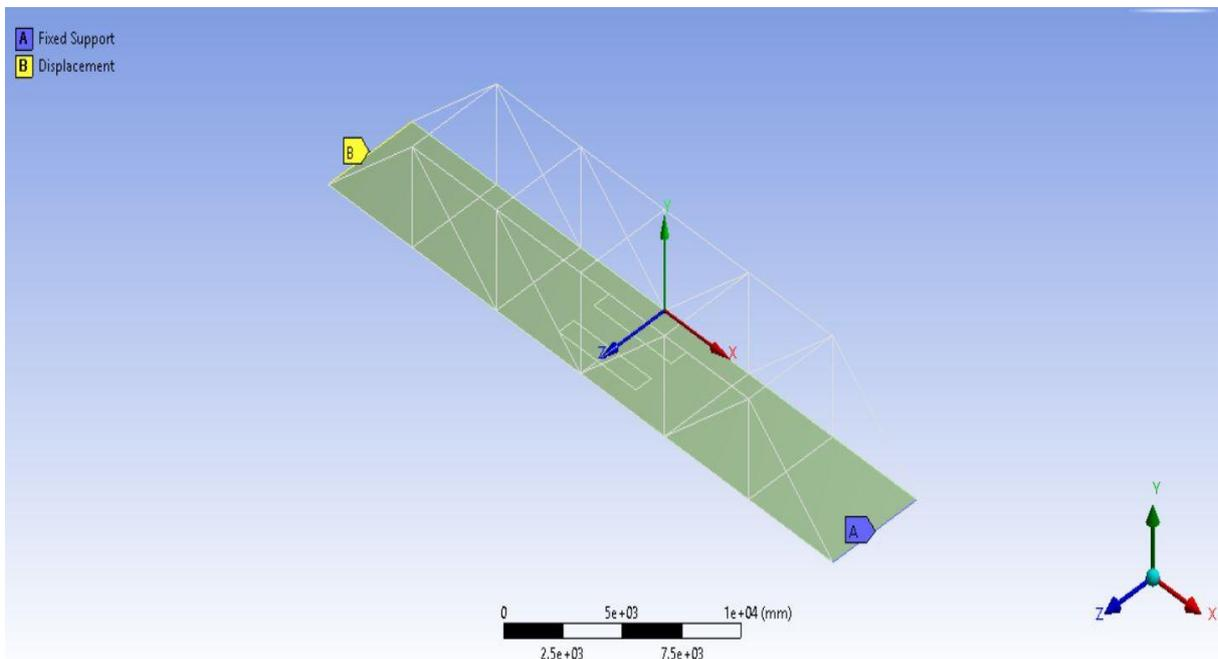
**Figure 3.16** Supports provided in Bridge in software
