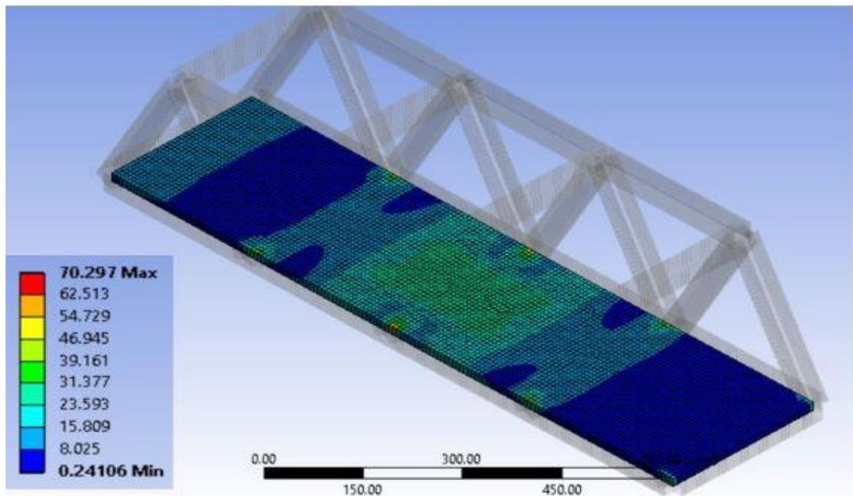
**Figure 4.2** Areas of Equivalent Stress according to the values
