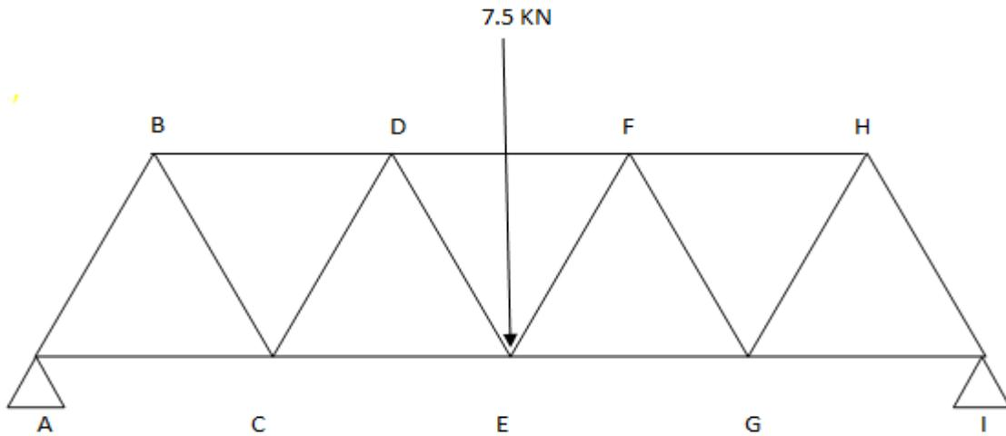
**Figure 4.12** Bridge geometry with location of load at the centre.
