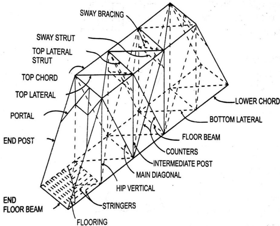
Figure 1.2 Components of a Truss Bridge<sup>[2]</sup> Source- Victor(2012)
