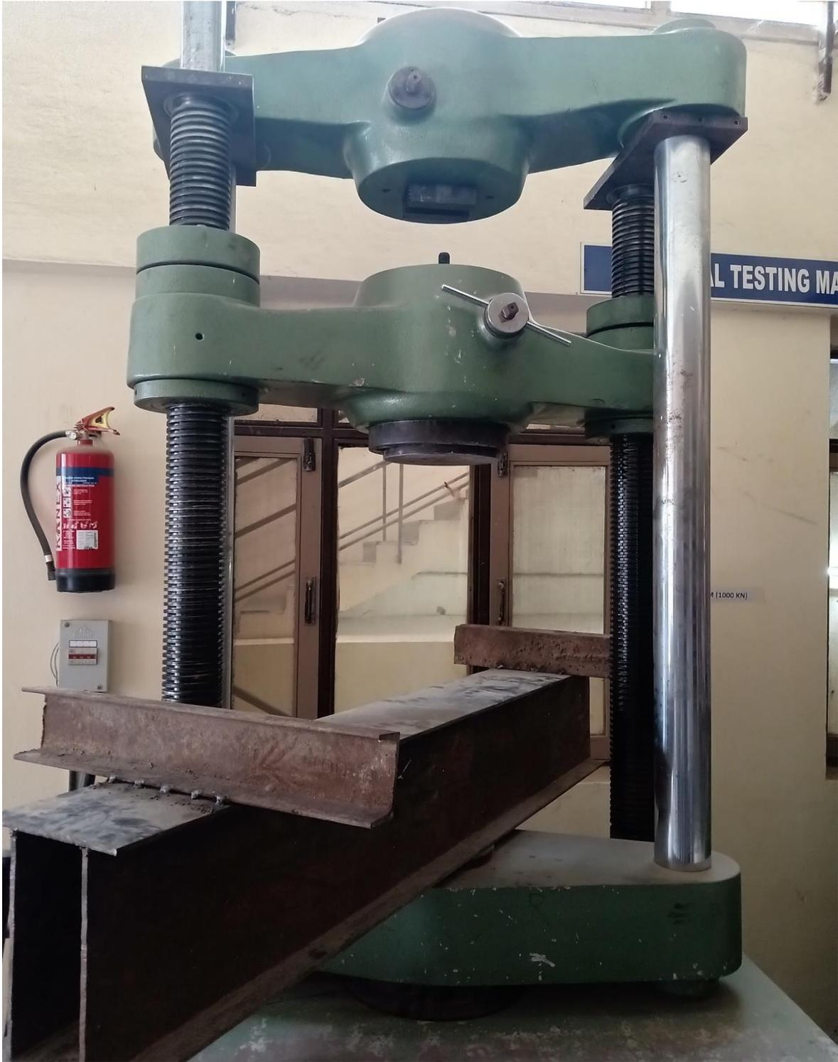
**Figure 3.19** Image of Universal Testing Machine.
