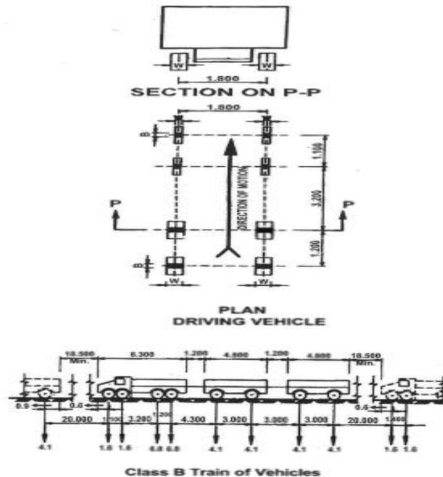
Figure 3.5 Class B loading Imprint Details<sup>[14]</sup> IRC-6 (2014)
