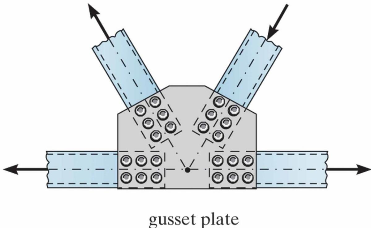
**Figure 3.8** Typical Truss Bridge joint<sup>[16]</sup>. Ponnuswamy(2014)
