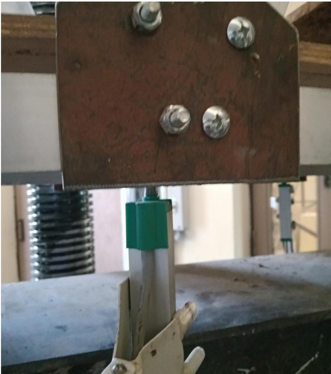
**Figure 3.20** LVDT attached at a node.
