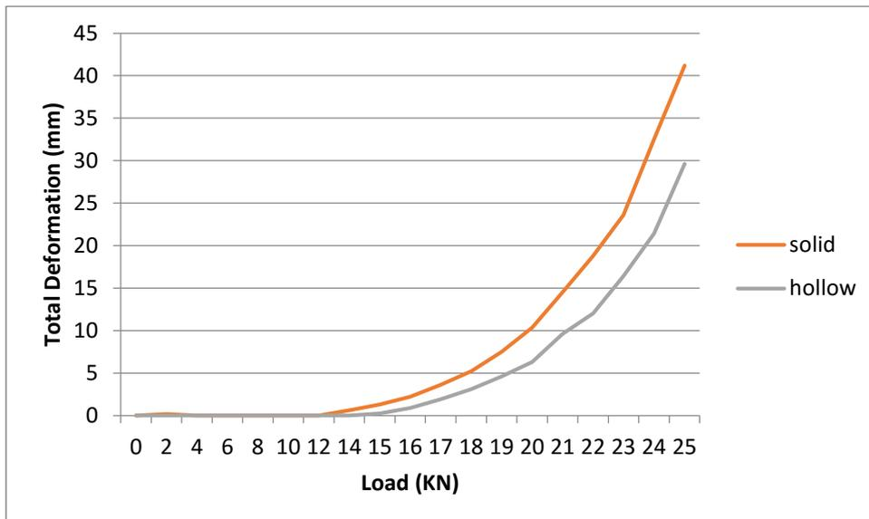
**Figure 4.11** Total Deformation comparison from the results collected from ANSYS.
