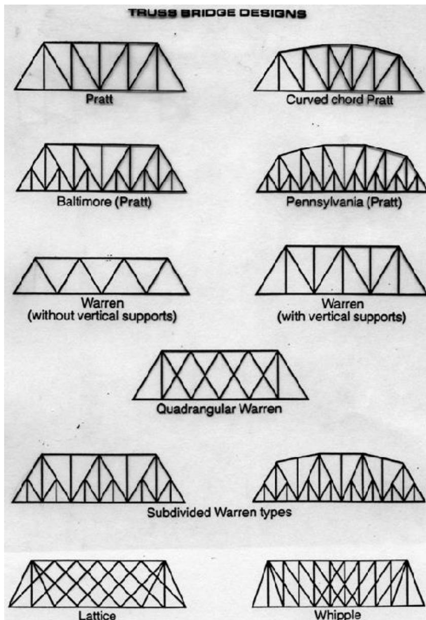
Figure 1.1 Typical Bridge Trusses<sup>[2]</sup> Source- Victor(2012)
