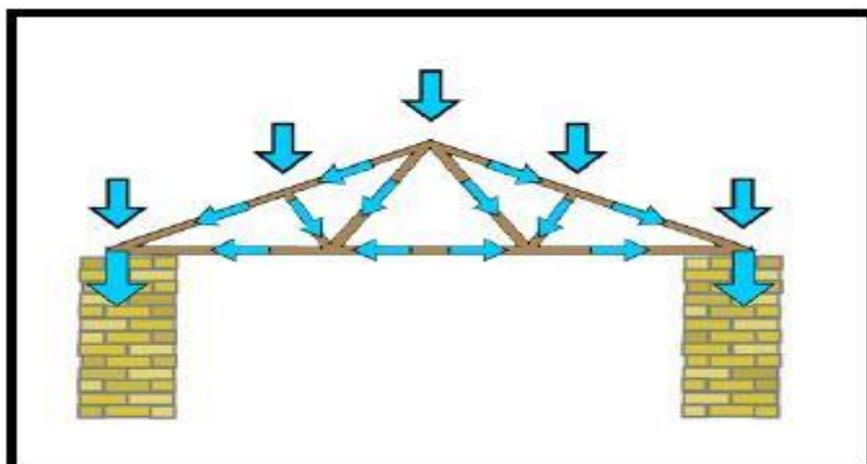
Figure 3.1 Distribution of load over a truss bridge<sup>[13]</sup> Source- Jasim(2016)
