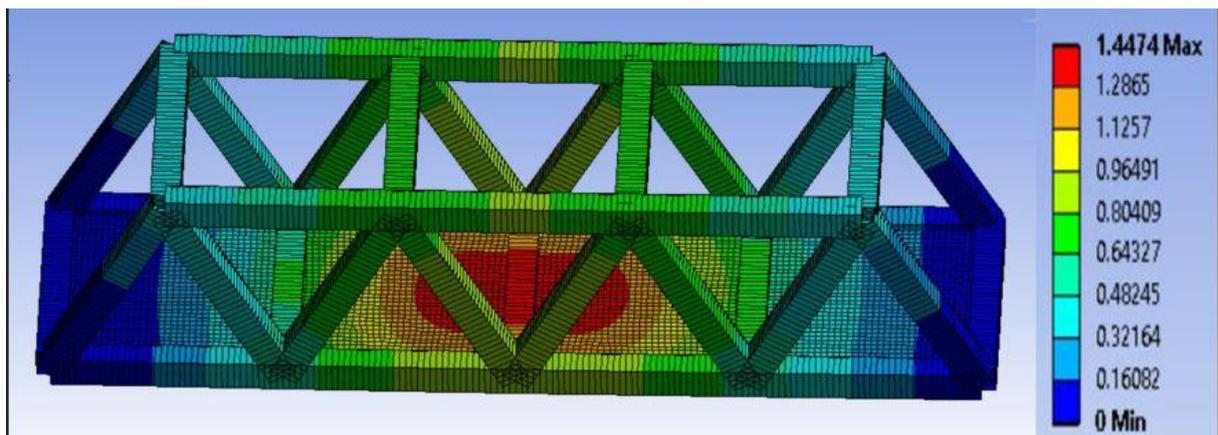
**Figure 4.1** Areas of Total Deformation according to the values.
