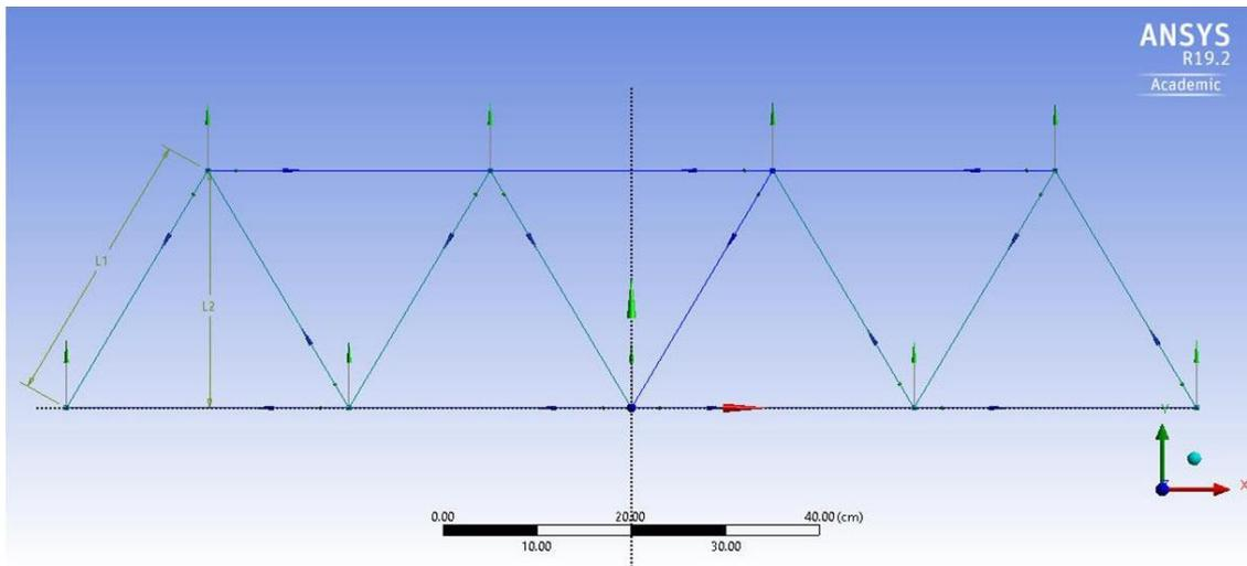
Figure 3.10 Line Body geometry of bridge.
