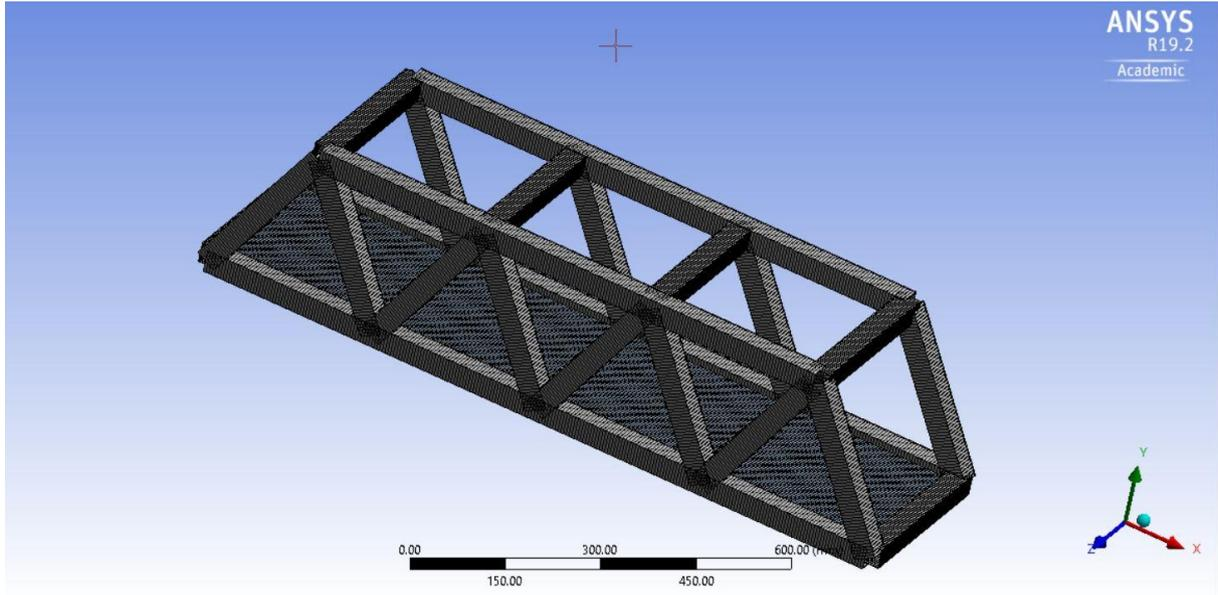
**Figure 3.15** Meshed Geometry of the bridge.
