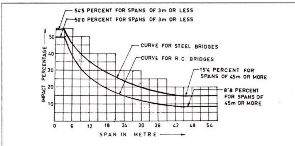
**Figure 3.6** Impact percentage Curve<sup>[14]</sup> IRC-6 (2014)
