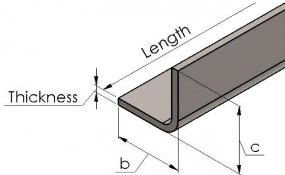
**Figure 3.9** Angle section view
