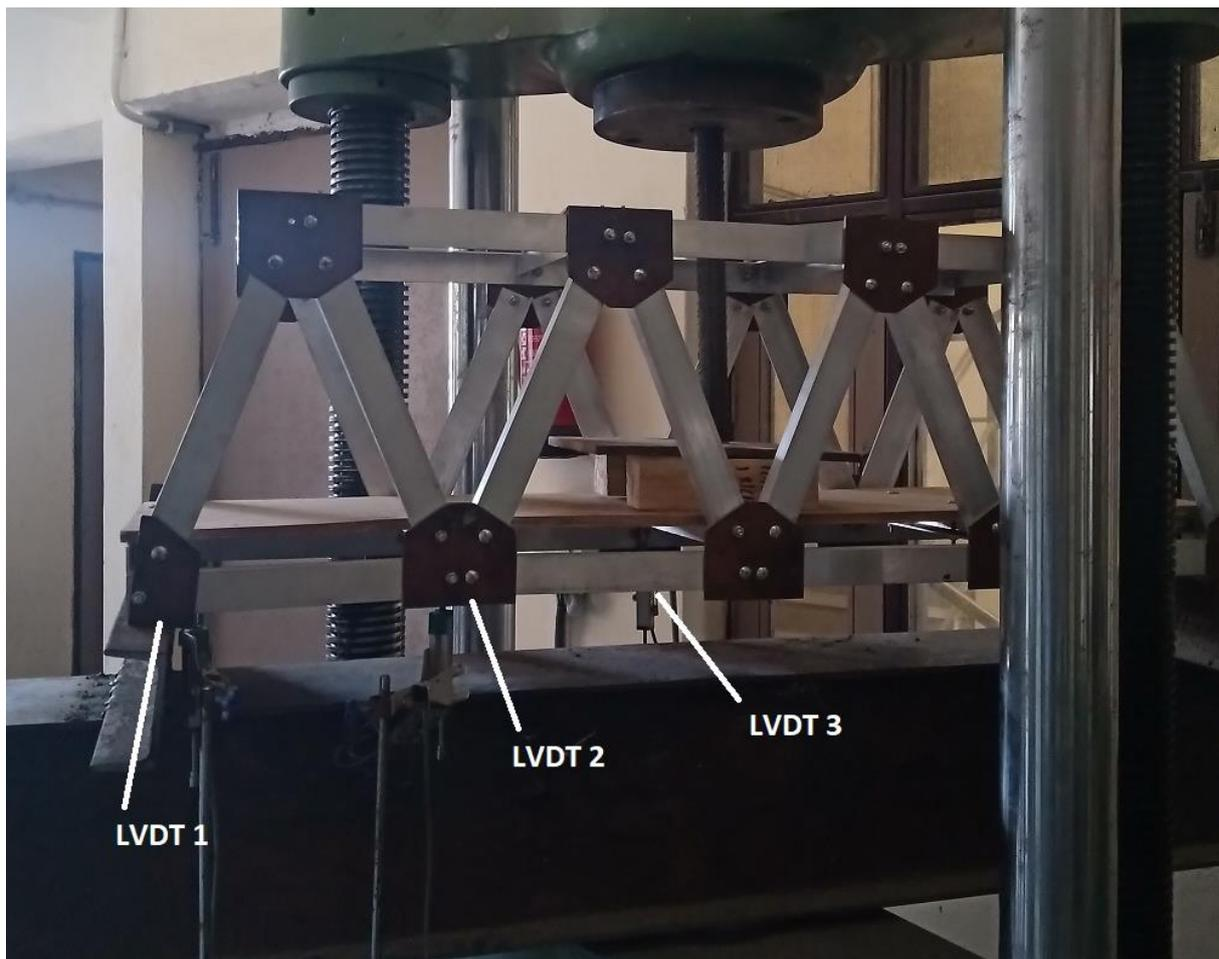
Figure 4.7 Locations of LVDTs
