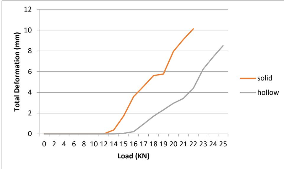
**Figure 4.10** Deformation comparisons at node 3 with respect to load
