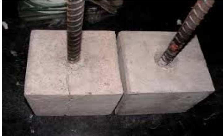
Figure 1.2 Reinforcement embedded in cubical mould
