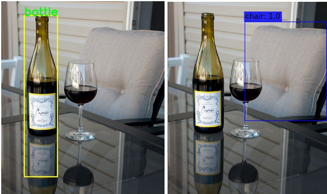
Fig 28: SDD(left) and YOLO(on right) outputs side by side
