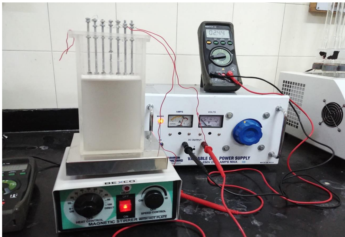
Figure B-1 Working of EC reactor
