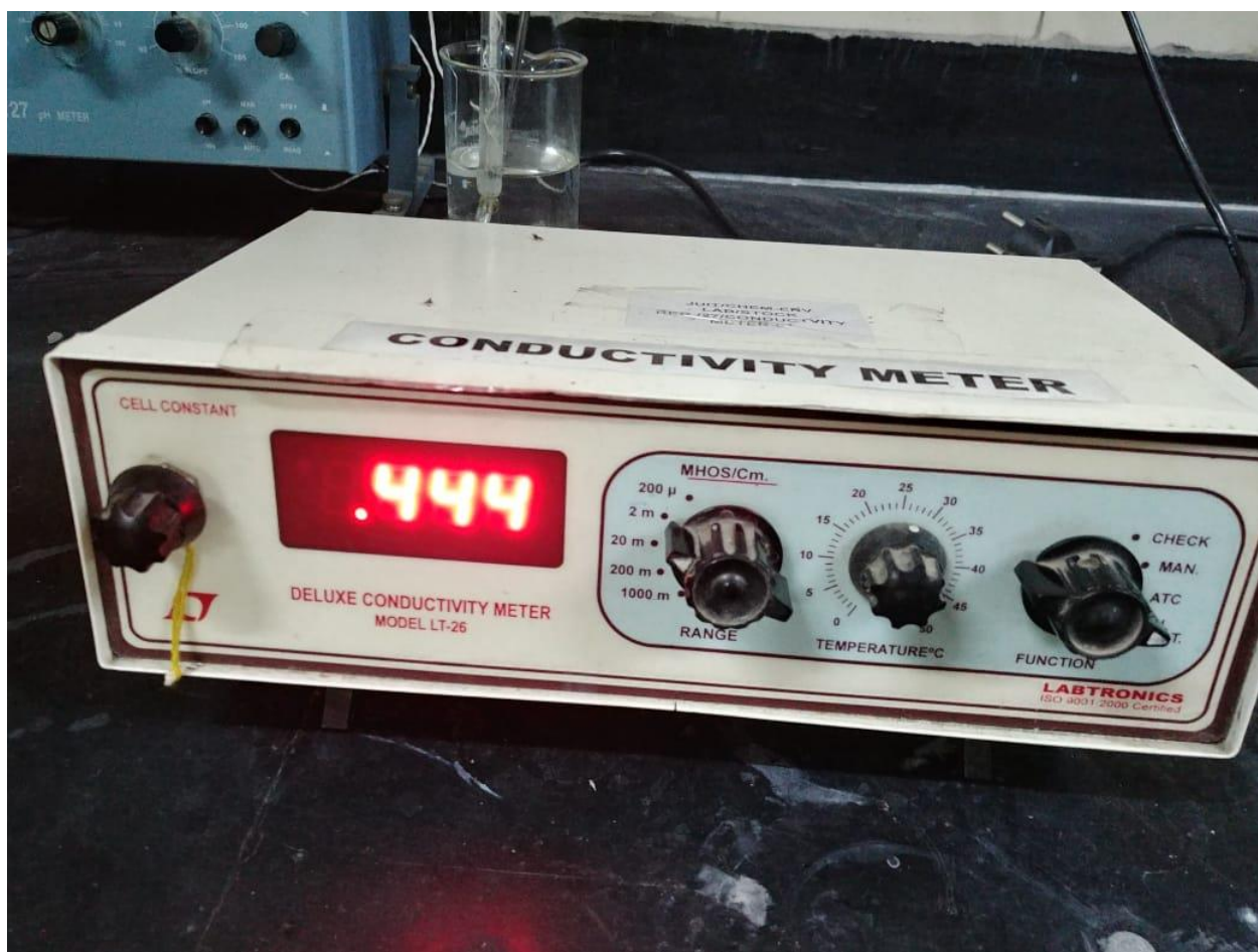
Figure B-7: Conductivity meter showing conductivity
