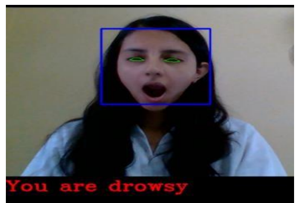
Fig 6.3(e): Yawning detected Fig 6.3(f): Yawning and small EAR detected
