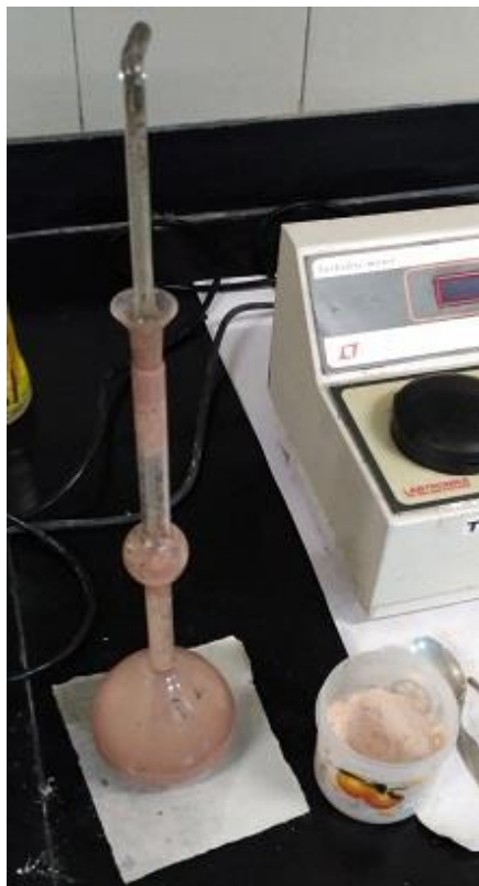
Fig 3.5 Le-Chatelier apparatus for calculation of Specific gravity
