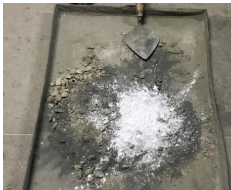
Figure 3.22 Dry mix of concrete with NS and MS
