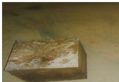
Figure 3.26 Sample after Acid attack
