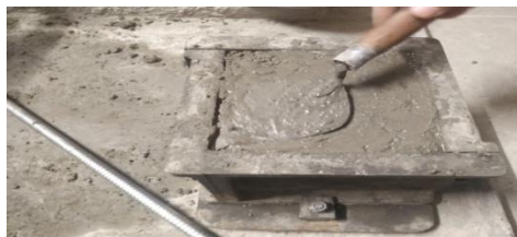
Figure 3.17 Filling mold with concrete
