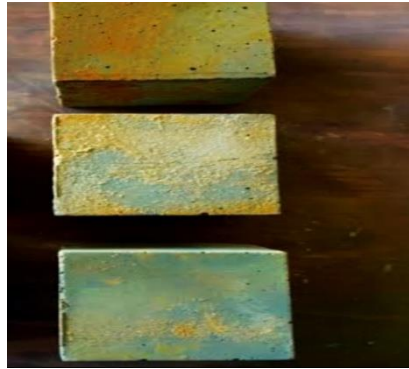
Figure 3.25 Samples after sulphate attack
