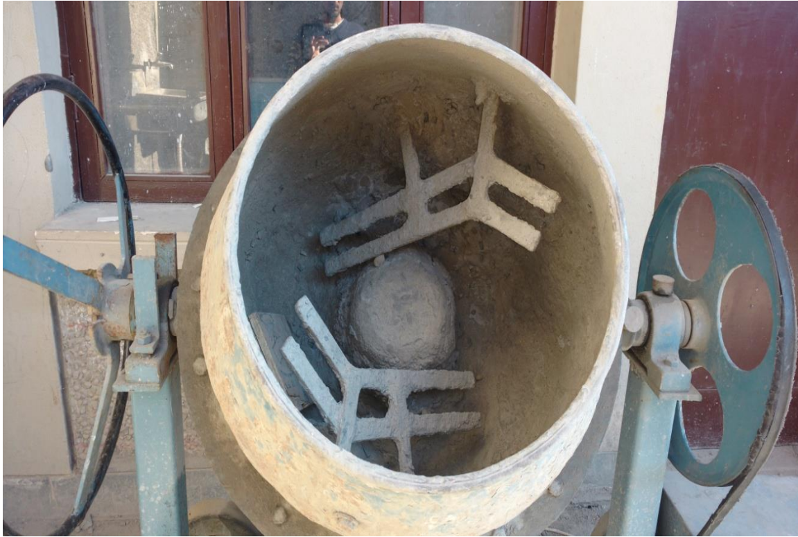
Figure 3.7: Concrete Mixing Machine.
