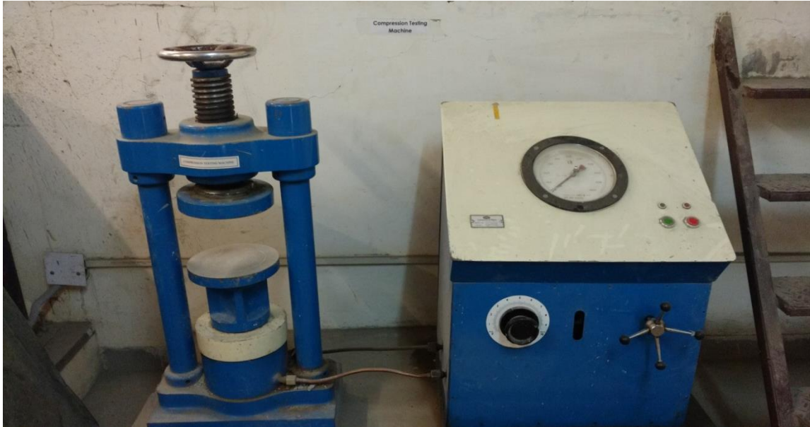
Figure 3.4: Compressive Testing Machine.
