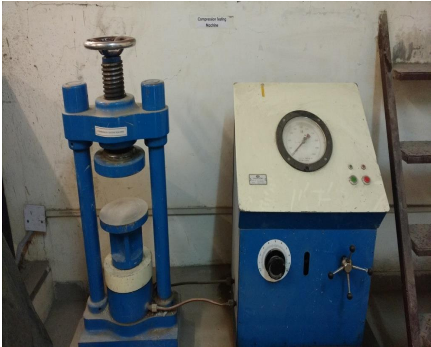
Figure 3.12: Compressive Testing Machine.
