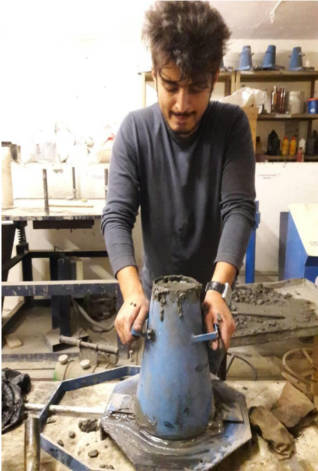
A9: Slump test
