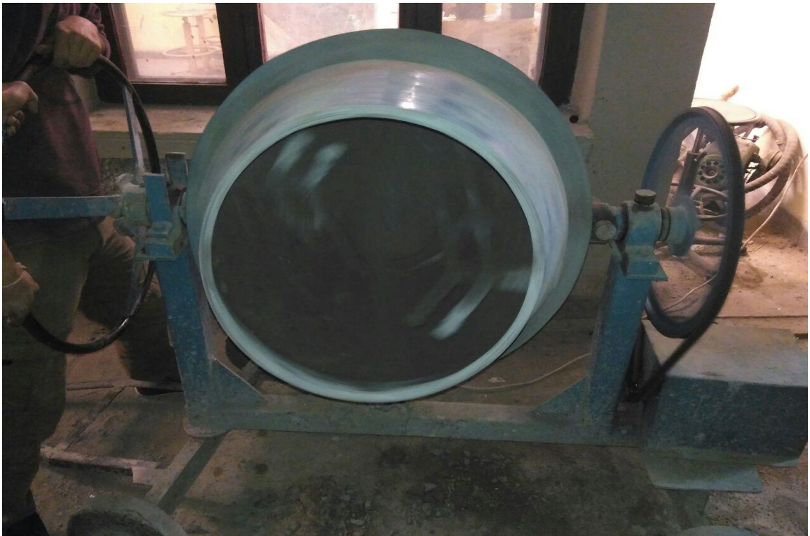
Figure.3.8:Mixer used for preparation of M30 samples
