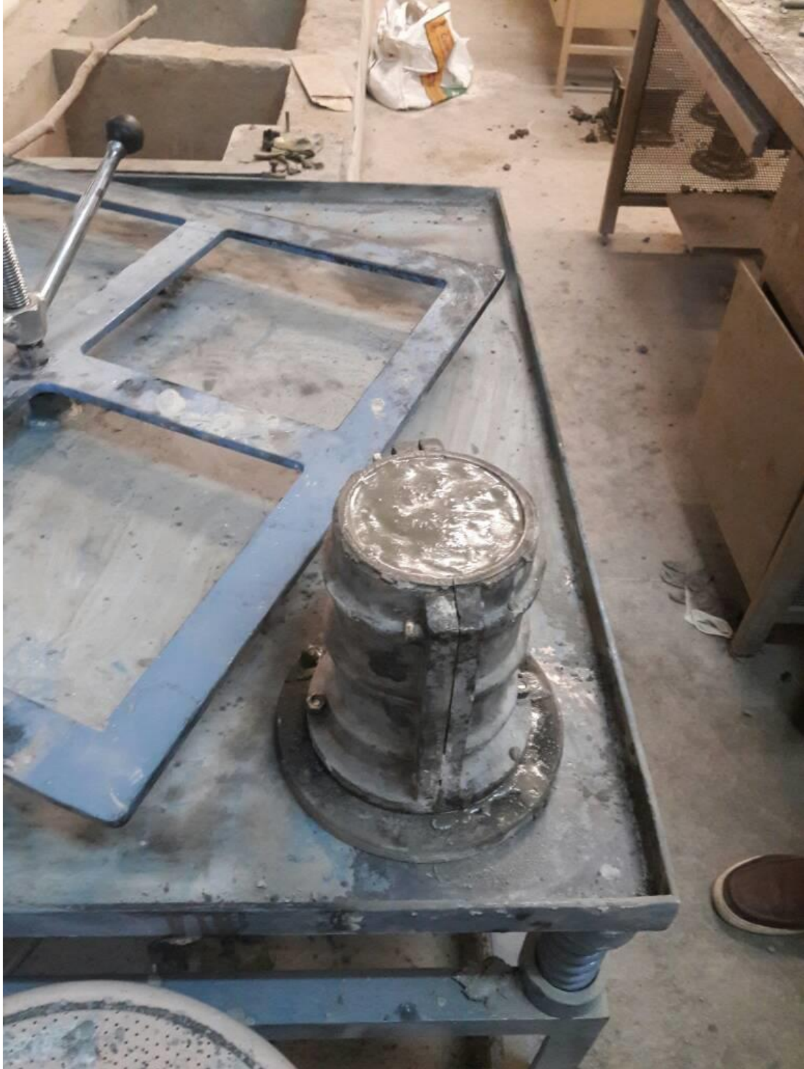
A6: Vibration being done on samples
