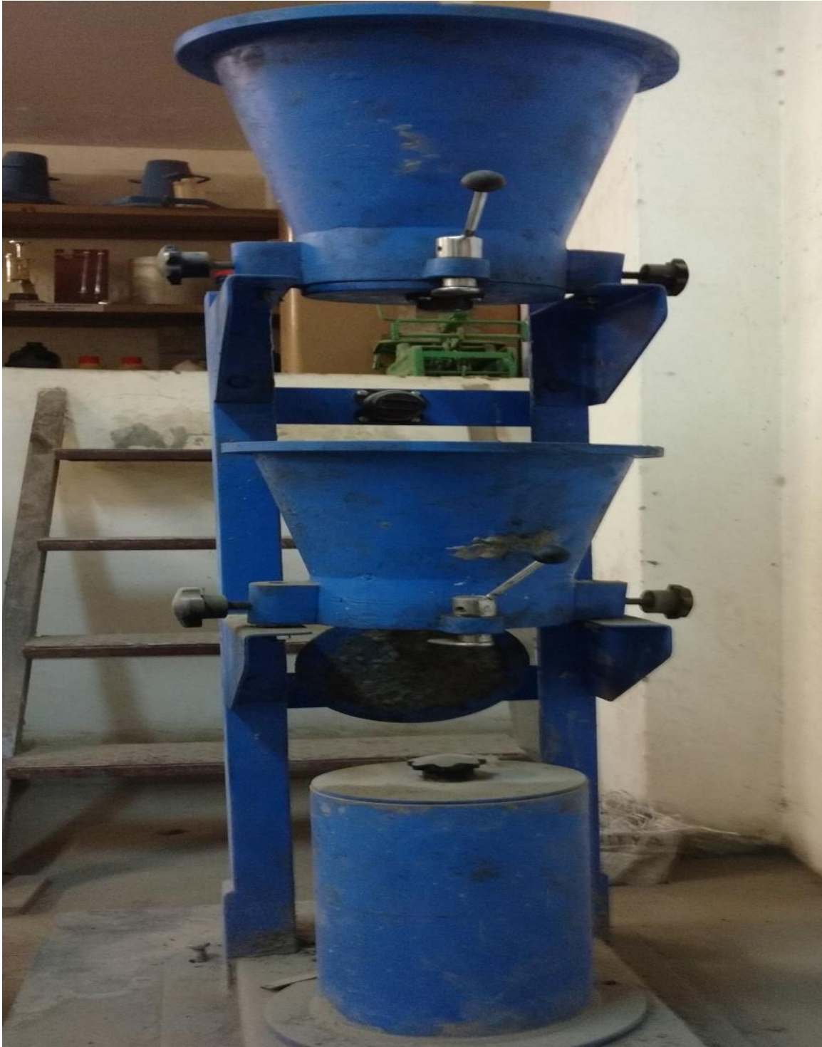
Figure 3.2: Compaction Factor Test
