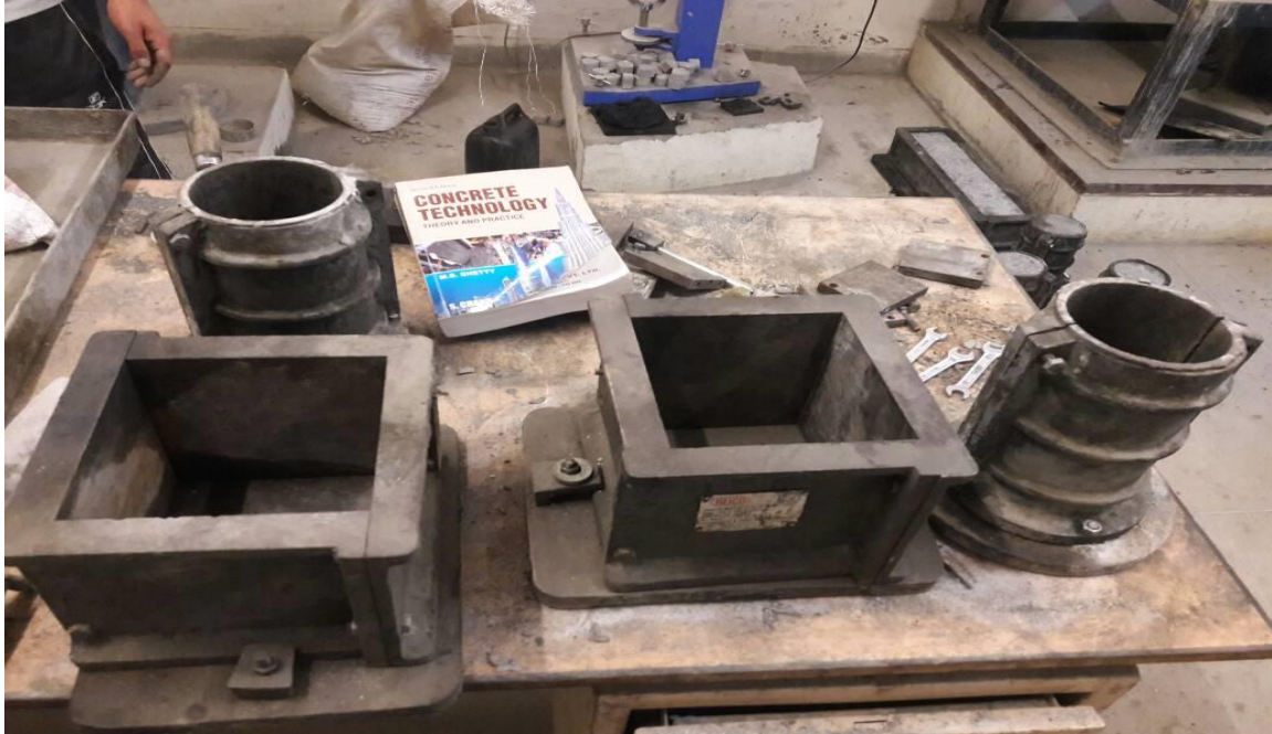
A3: Cylinder and cube moulds
