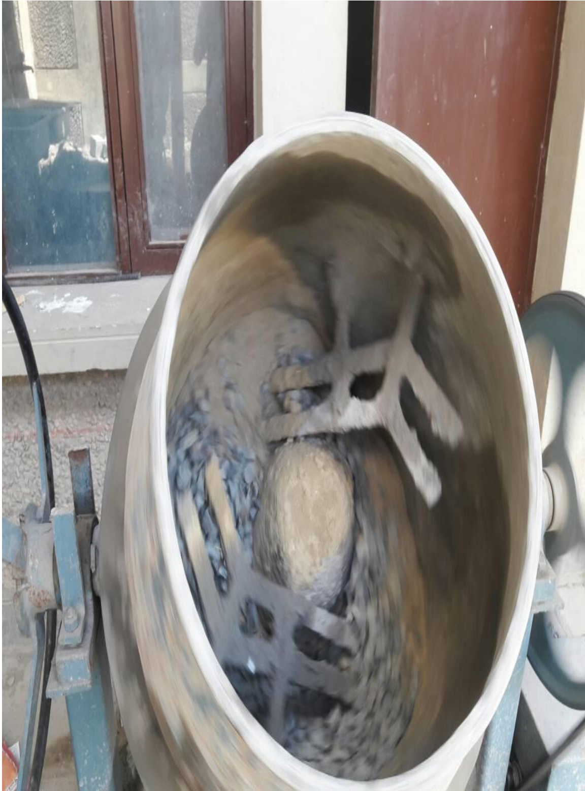
A5: Mixer used for preparation of M30 mix
