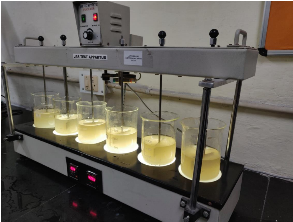
Figure 9: Jar Test Apparatus for Optimum Coagulant Dosage
