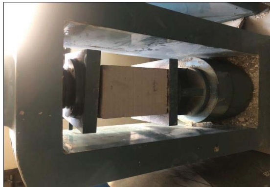
FIG 10- AAC block for submerged in water. FIG 11: AAC block tested under UTM.
