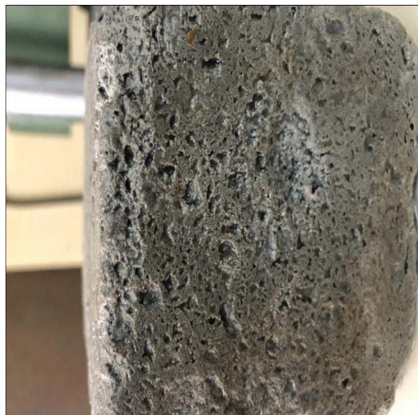
FIG15-AAC block having low alumina content
