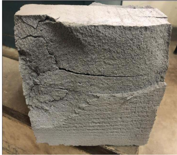
FIG 13: AAC block Failure Pattern
