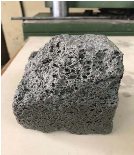
FIG14- AAC block having high alumina content
