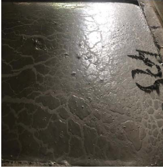
FIG 5- Casted AAC in mould.
