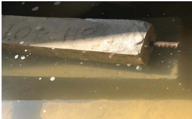
FIG 10- AAC block for submerged in water. FIG 11: AAC block tested under UTM.
