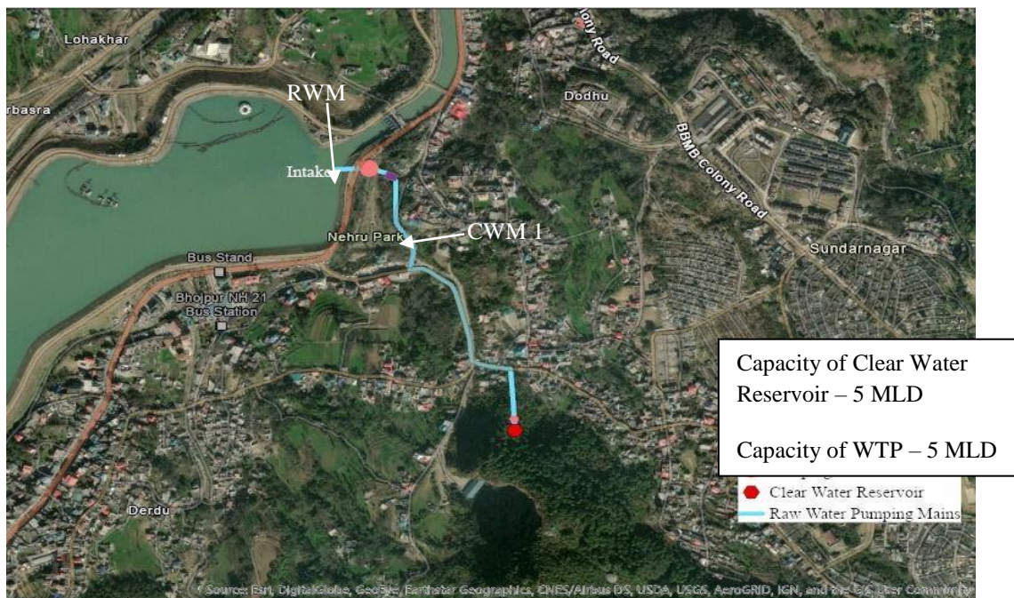
Figure: 4.6 Layout of WTP, Pumping Stations, Clear Water Reservoir and Raw Water Pumping Mains
