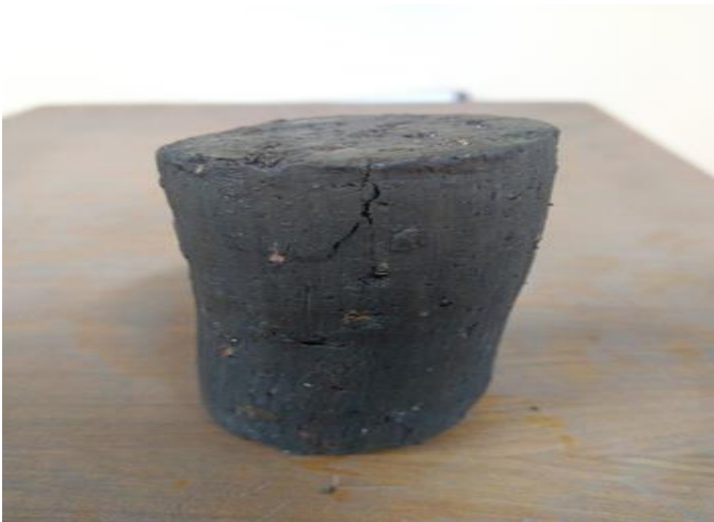
Fig 5.2.4 An UCS Sample failed while testing.
