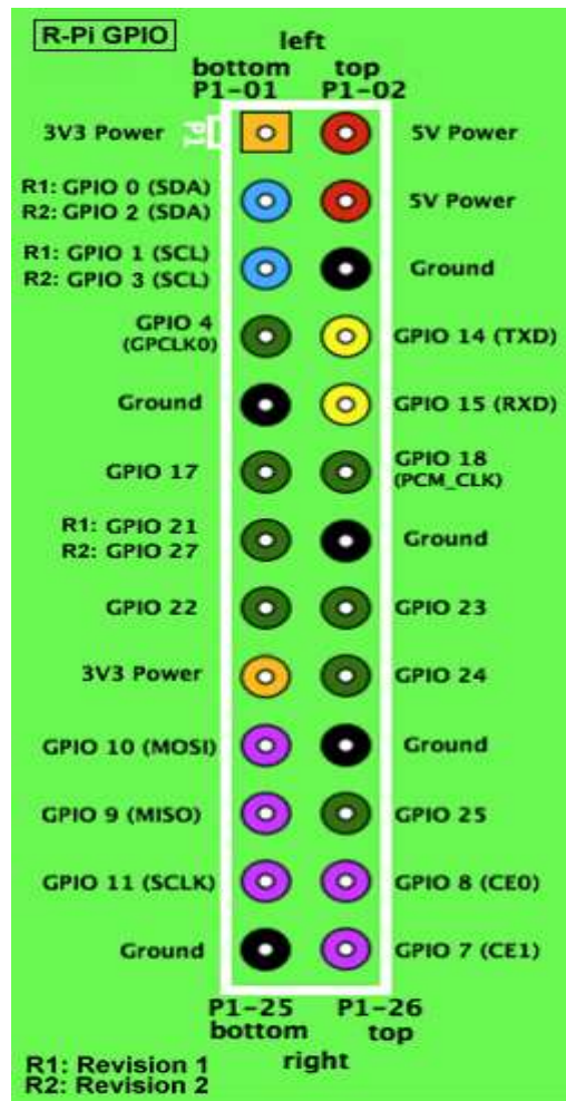
Figure 3.2 - Pin configuration of Pi
