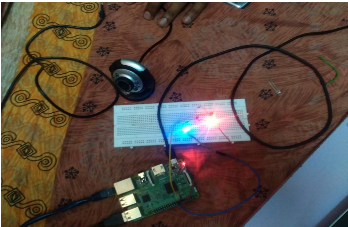
Fig. 4.3 LEDs switched ON when Bulb and Fan detected
