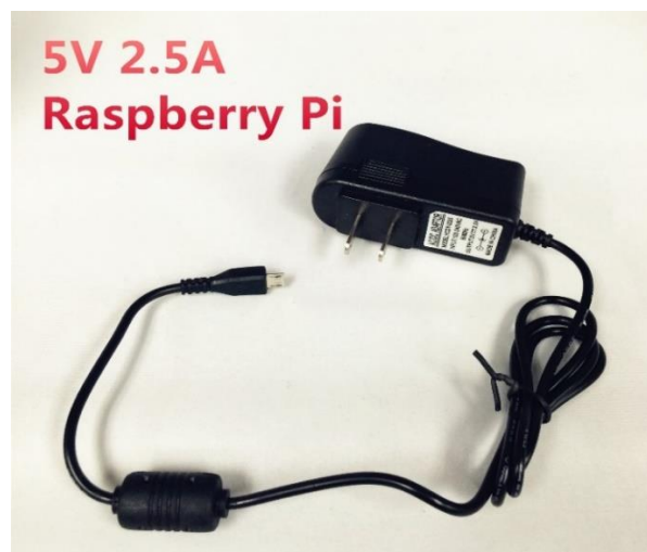
Fig 1.2 Power supply used to power raspberry pi 3
