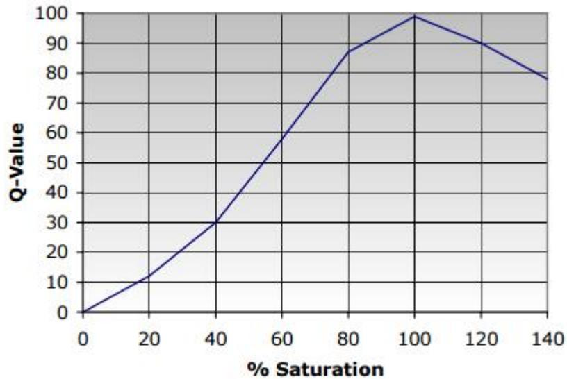
**FIGURE 6.29: Q-VALUE CHART FOR DISSOLVED OXYGEN**
