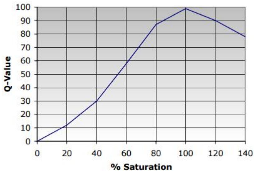
**FIGURE 6.11: Q-VALUE CHART FOR DISSOLVED OXYGEN**
