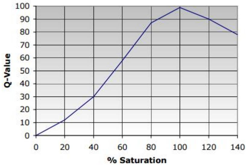
**FIGURE 6.2: Q-VALUE CHART FOR DISSOLVED OXYGEN**
