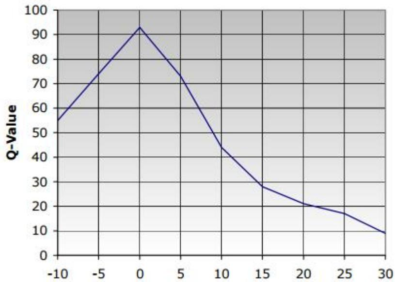
**FIGURE 6.35: Q-VALUE CHART FOR TEMPERATURE**
