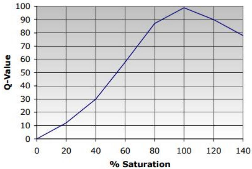
**FIGURE 4.1: Q-VALUE CHART FOR DISSOLVED OXYGEN**
