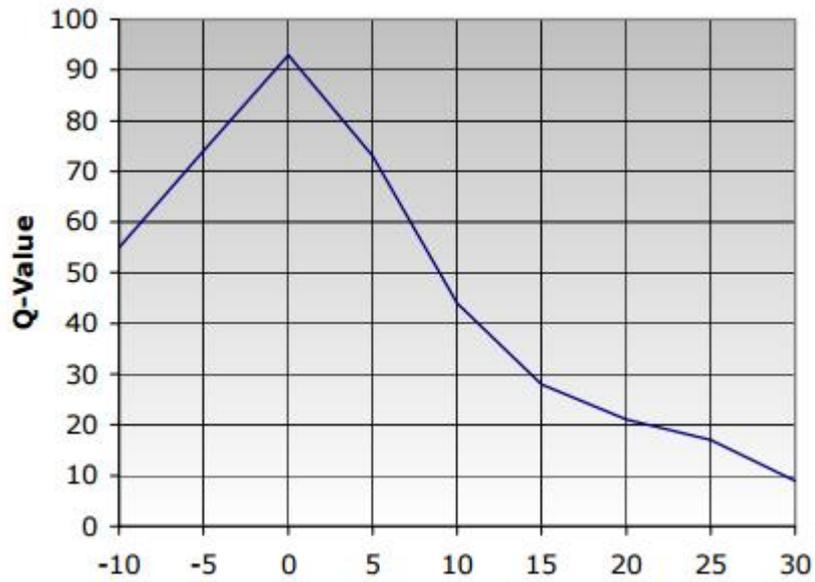
**FIGURE 6.26: Q-VALUE CHART FOR TEMPERATURE**
