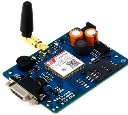
Figure 4.3: GSM module(SIM 800A Quad Band GSM)
