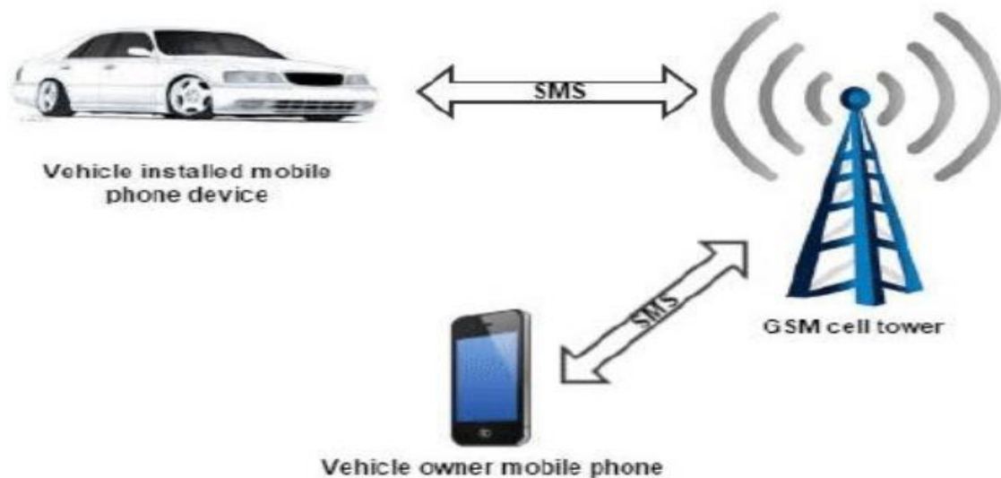
Figure 3.1 Architecture of vehicle theft alert system
