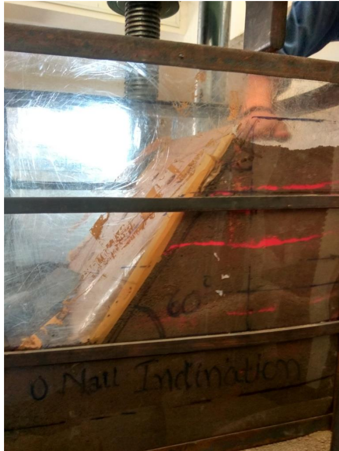
FIG 3.11 Preparation of 60° Slope
