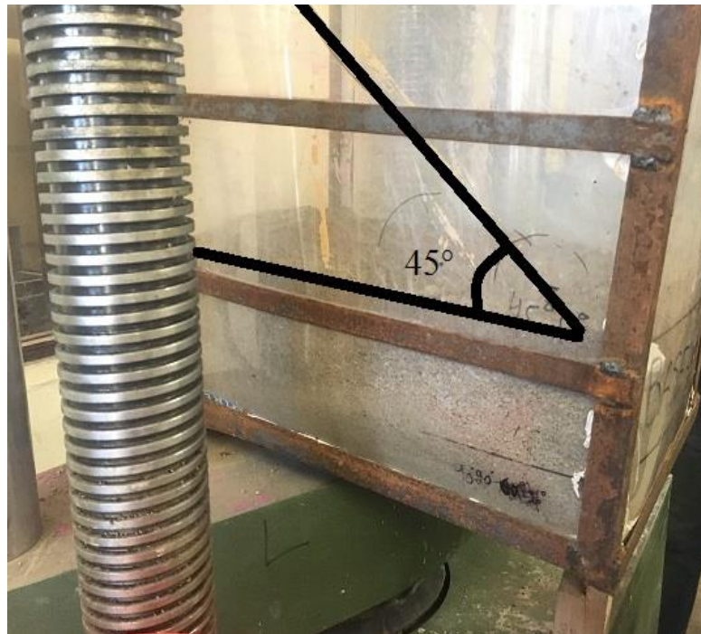
FIG 3.10 Preparation of 45° Slope
