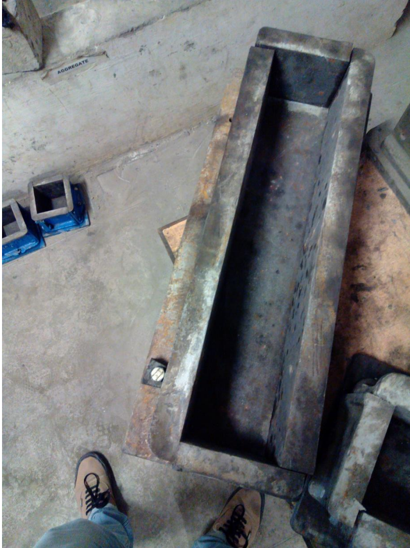
Beam specimen mould(150mmX150mmX150mm)
