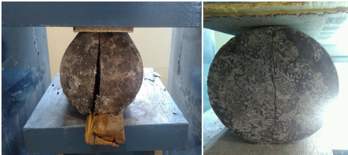
Fig no 3.8 Split tensile test on cylinder
