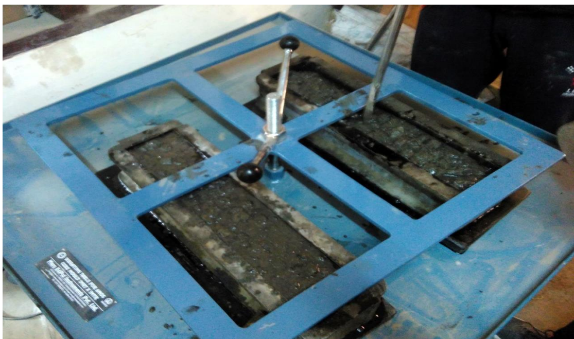
Fig no 3.5 Casting of specimens
