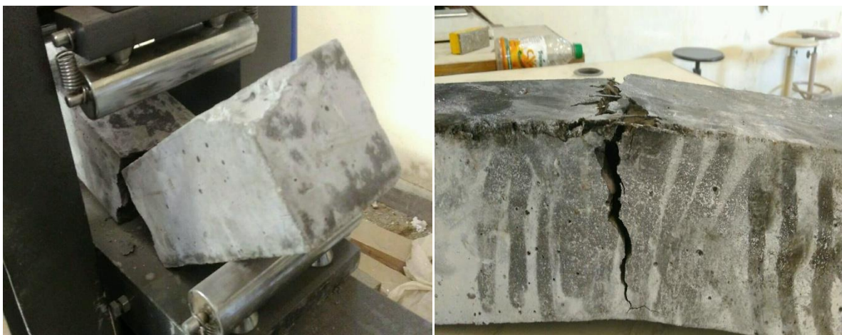
Fig no 3.7 Flexural test on beam
