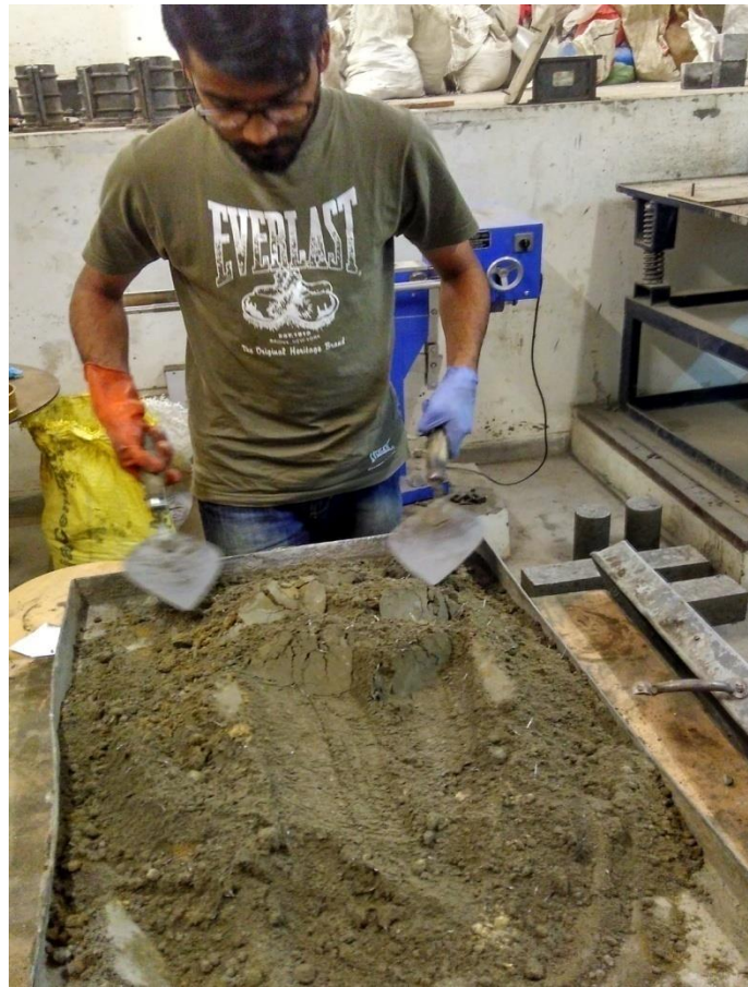
Fig no 3.3 Hand mixing of specimen
