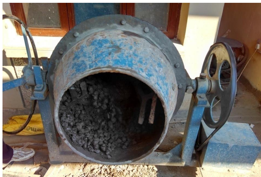
Fig no 3.4 Machine mixing of specimen
