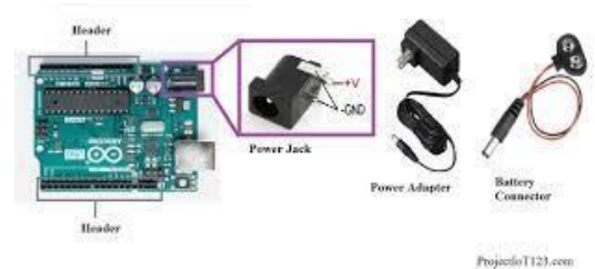
Fig.6. Power supply components
