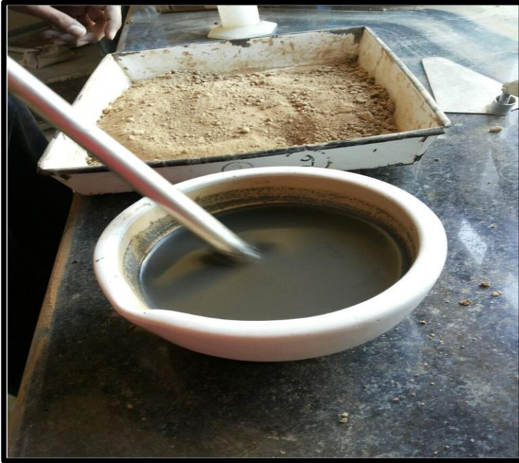
MAKING OF CEMENT SLURRY
