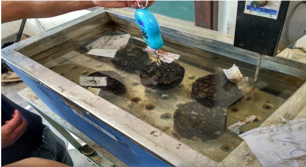
Fig.4.12: - Curing of Cores and Weight measurement
