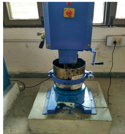
Fig.4.8:- Mixing of Aggregate with Bitumen
