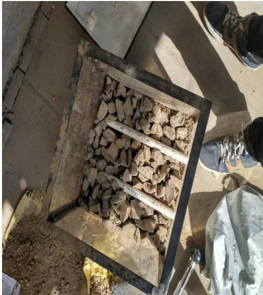
Fig.6.3.: -Provision of pipes for water outlet
