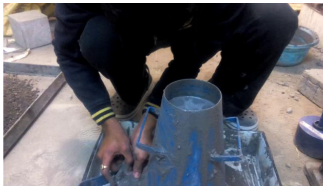
SLUMP FLOW TEST IN PROGRESS
