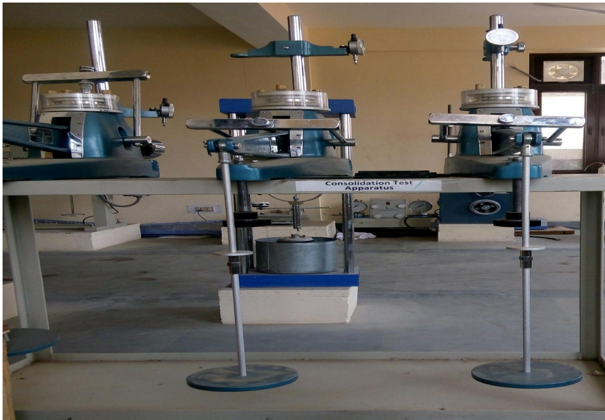
Fig.-5 (Setup for Swelling test)
