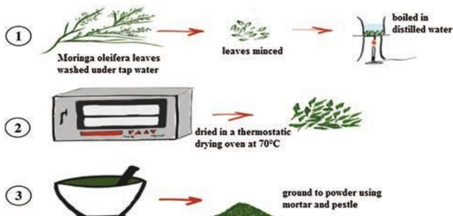
Fig 3.1 : Steps to make powder of the leaf to be used for extraction
