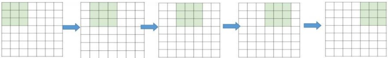
Fig 2.5: For Stride = 1, the filter moves once for each connection
