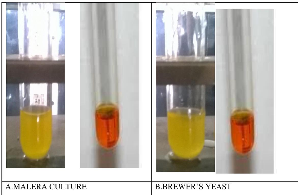
**FIG 16 Qualitative test for ethanol production in juice fermentation**
