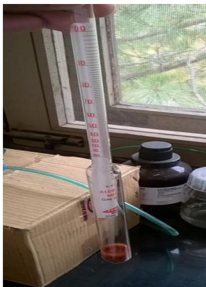
**FIG 6 Pictorial representation of alcohol-meter**
