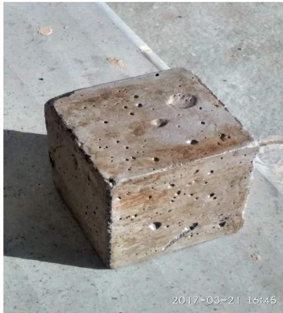
Figure 4.10 – water resistance on filler based MOC cube
