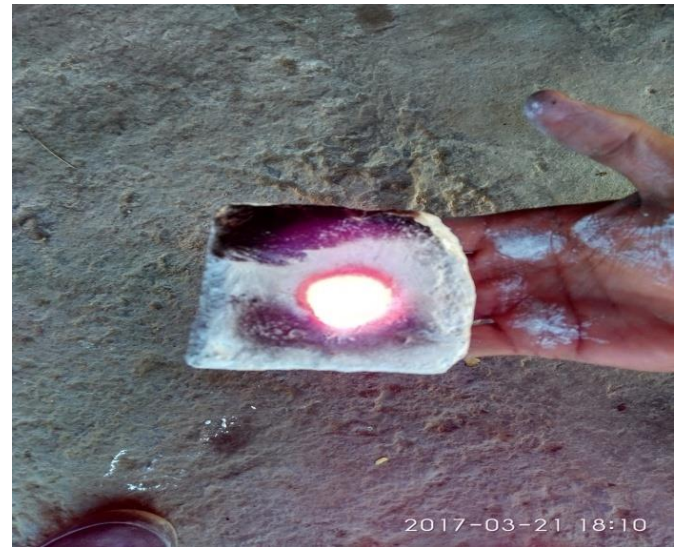
Figure 4.11 – Fire resistance test on pure MOC cubes
