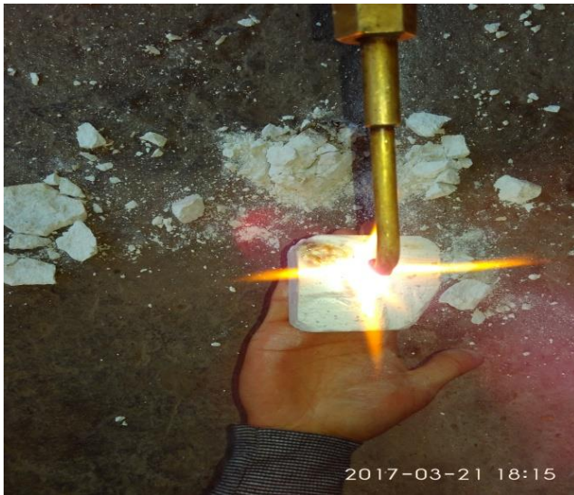
Figure 4.11 – Fire resistance test on pure MOC cubes
