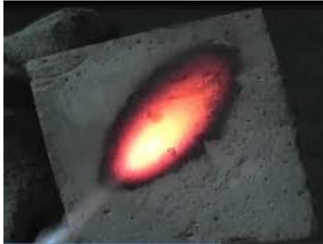
Figure 4.12 – Fire resistance test on cement cube
