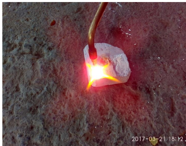
Figure 4.12 – Fire resistance test on filler based MOC cube
