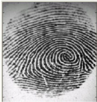
Fig. 2 Fingerprint image acquired by an Optical Sensor.
