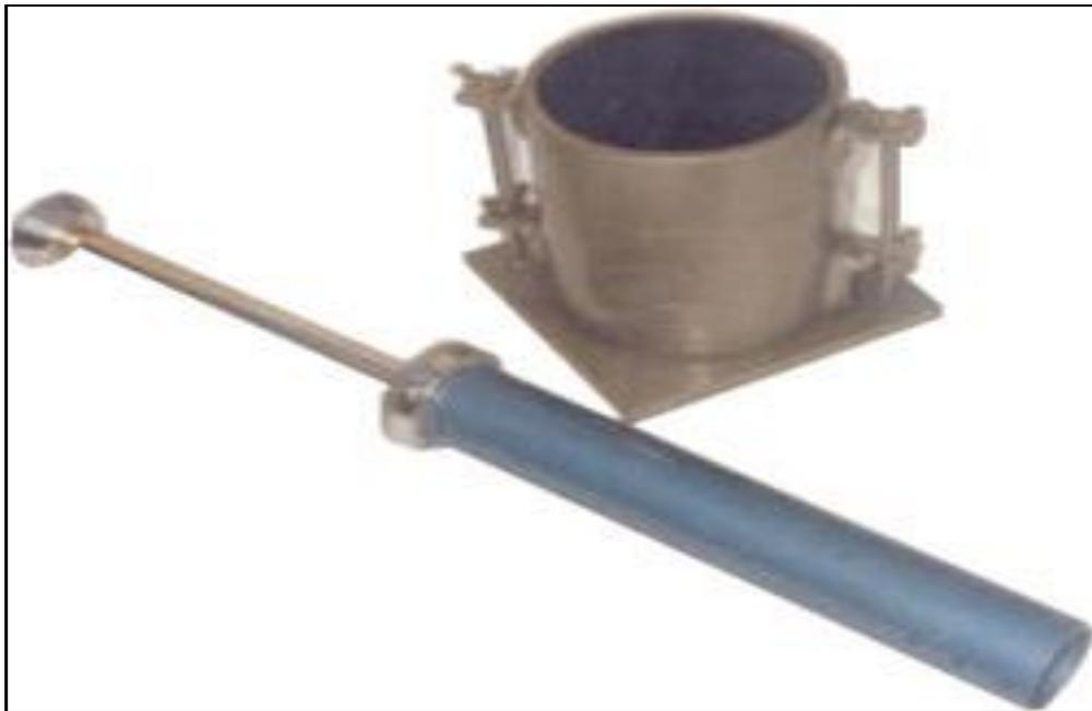
Fig 3.3 Procter test apparatus
