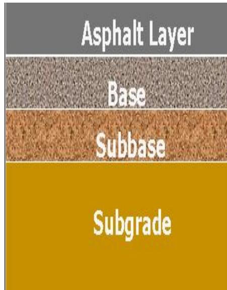
***FIG 1.1(A) Flexible Pavement***
