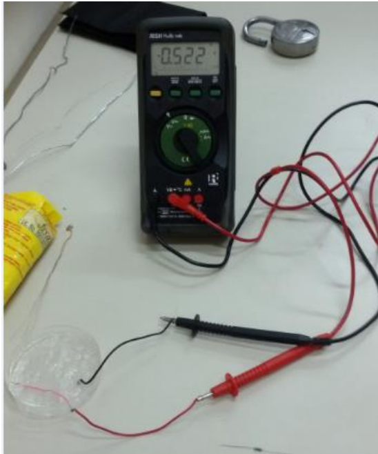
Figure 2.6. Paper clip-Copper wire thermocouple in ice
