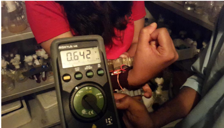
Figure 4.5 Measuring voltages from the combination of four TEGs.
