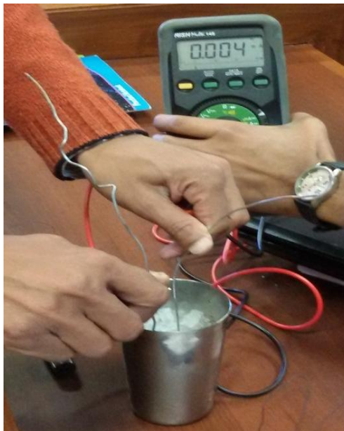
Figure 2.5 : Iron aluminum thermocouple with one junction in ice.
